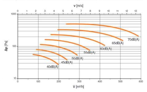
Volumetric flow V Air velocity v Pressure loss Δp
